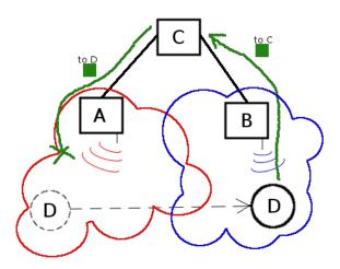
**Figure 1:** Hand-over with B.A.T.M.A.N. The moving Client 'D' will immedtiatly send the packets through the correct route, while Node 'C' will still use the wrong route until it will receive the new OGM from B
